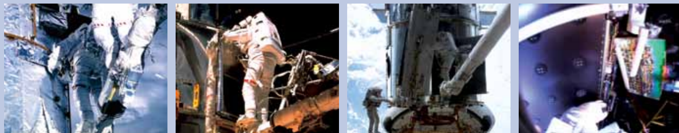
Figure 1.8 – HST Servicing Sophistication Progression – Servicing the Hubble Space Telescope demanded more than replacing hardware that was designed to be serviced. As unexpected issues arose during the past 20 years of the mission, many tasks required developing innovative techniques to solve specific problems. From left to right: First, the repair of the light shield during SM2. Second, the installation of the New Outer Blanket Layer during SM3A. Third, the attachment of the NICMOS Cooling System external radiator during SM3B. Last, the card removal for the Advanced Camera for Surveys Repair during SM4. Each repair required accessing interfaces that were not designed for servicing, and each was fully successful.
