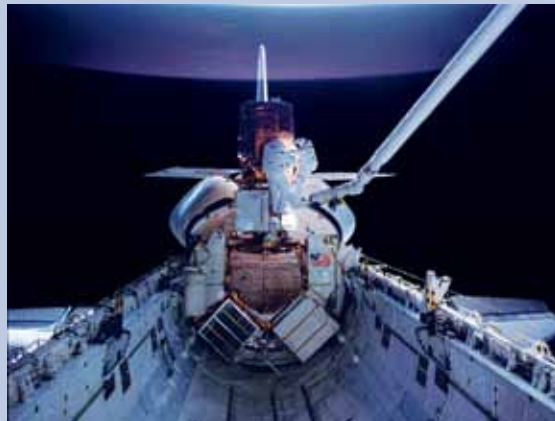
Figure 1.5 – Solar Maximum Mission in the Space Shuttle Bay – The Solar Maximum Mission was one of the first orbiting spacecraft to be retrieved, repaired, and redeployed using satellite servicing. This photograph from 1984 shows the spacecraft being repaired by astronauts in the payload bay of the space shuttle Challenger.
