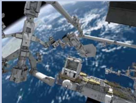
Figure 4.12 – Dextre Pointing Package (DPP) – This rendering shows the DPP hardware being used on the International Space Station for Earth observations. This hardware will demonstrate fine pointing of the robotic arm using algorithms developed to support robotic servicing operations.
