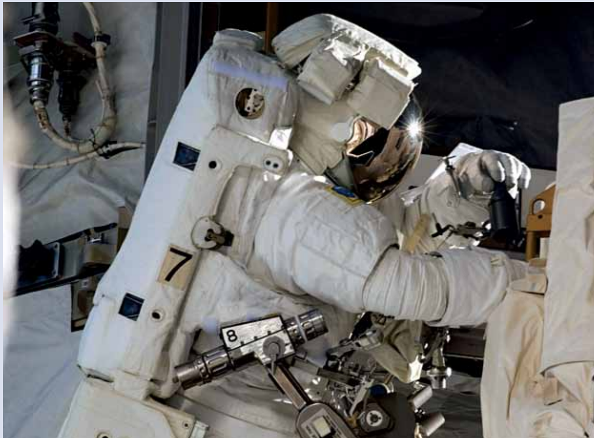
Figure 4.13 – Astronaut in Action – Astronaut Ron Garan, STS-124 mission specialist, participates in the mission’s third scheduled session of Extravehicular Activity (EVA) as construction and maintenance continue on the International Space Station (ISS). During the six-hour, 33-minute spacewalk, Garan and astronaut Mike Fossum (out of frame), mission specialist, exchanged a depleted Nitrogen Tank Assembly for a new one, removed thermal covers and launch locks from the Kibo laboratory, reinstalled a repaired television camera onto the space station’s left P1 truss, and retrieved samples of a dust-like substance from the left Solar Alpha Rotary Joint for analysis by experts on the ground. The ability to perform such feats on-orbit provides the inspiration for developing the art of satellite servicing.
