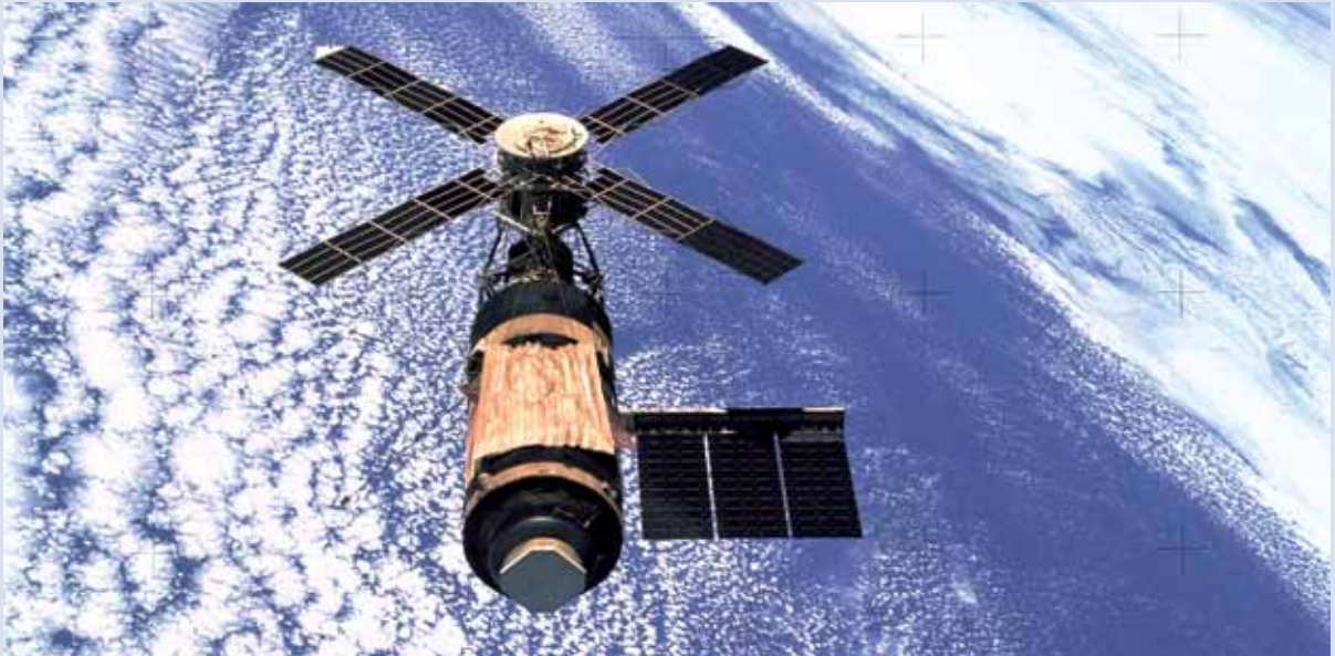
Figure 1.4 – The Repaired Skylab – Launched in 1973, Skylab was not only NASA's first space station, it was also the Agency's first human satellite servicing endeavor. A successfully deployed parasol (seen on the top of the central cylinder of the spacecraft, nearer to the viewer) restored an acceptable thermal configuration and saved the mission.
