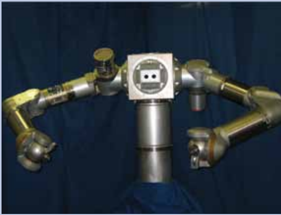
Figure 4.6 – Ranger Telerobotic Shuttle Experiment – The Ranger dexterous manipulator pair mounted to a head that is attached to a positioning leg. This hardware was designed to be positioned at a worksite using a grapple arm or a positioning leg.
