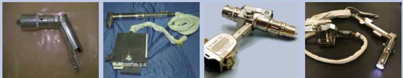
Figure 1.12 – EVA Power Tool Progression – Astronaut servicing tools have progressed as the complexity of servicing tasks has increased. Shown here is a series of EVA power tools—torque-producing, battery-powered, bolt-turning drivers—developed over the course of the space shuttle and ISS Programs. From left to right: the original shuttle Mini Power Tool is a low torque, household screwdriver with limited capacity and reliability. The Power Ratchet Tool was developed for the HST Deployment Mission to provide high-torque and long battery life, and continued in service for all HST Servicing Missions. The Pistol Grip Tool was developed jointly between the HST and ISS Programs, as both were in need of a medium-torque, highly accurate, and self-contained tool for precision and construction tasks. The Mini Power Tool was developed for HST Servicing Mission 4 as a high-speed, high-precision, illuminated dexterous screwdriver capable of removing hundreds of tiny fasteners.
