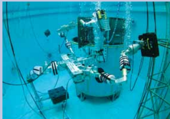
Figure 1.16 – Robotic Assistants – An astronaut in a simulated spacesuit is assisted during notional satellite servicing tasks by two robotic manipulators: one helping to open/hold the door while the other one stows an old battery and grabs a replacement. A free-flying camera platform observes the operation and captures this photograph.
