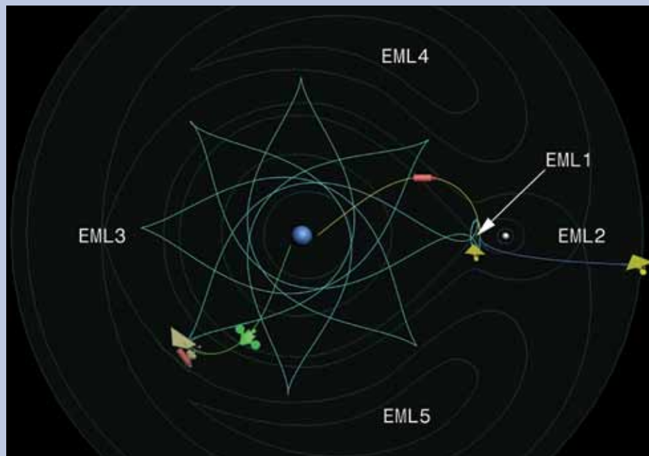
Figure 4.8 – The LOTUS – This figure depicts the LOTUS in the context of the mission sequence for Notional Mission 5. The robotic servicing vehicle travels to a Lyapunov orbit about Earth-Moon L1 (top center red cylinder), where the large telescope later arrives from Sun-Earth L2 to be captured. After the servicer and telescope are joined (lower left yellow/red spacecraft), they insert into the LOTUS with a very small \Delta V and are later met by the crew vehicle (lower left green spacecraft). The crew vehicle, robotic servicer, and telescope remain together on the LOTUS until servicing of the telescope is complete, at which time the crew vehicle deorbits. The LOTUS proceeds to naturally carry the servicer and telescope back to L1, where the servicer will reinsert into the Lyapunov orbit for long-term station-keeping. The telescope performs a small maneuver to exit the Earth-Moon system and return to its operational orbit about Sun-Earth L2 (right).
