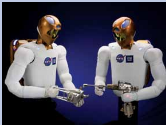
Figure 1.11 – Robonaut 2 – A "human equivalent" robot, Robonaut 2 (R2), handles tools similar to the ones it will use after its deployment to the International Space station in early 2011.
