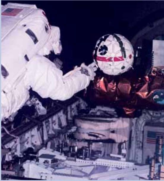
Figure 1.15 – AERCam Sprint – Autonomous Extravehicular Activity Robotic Camera Sprint (AERCam Sprint) in the cargo bay of the Earth-orbiting space shuttle Columbia during STS-87. The AERCam Sprint is an experiment that demonstrates using a free-flying video camera for remote inspections. It is a 14-inch diameter, 35-pound sphere that contains two video cameras, an avionics system, and 12 small Nitrogen gas thrusters.
