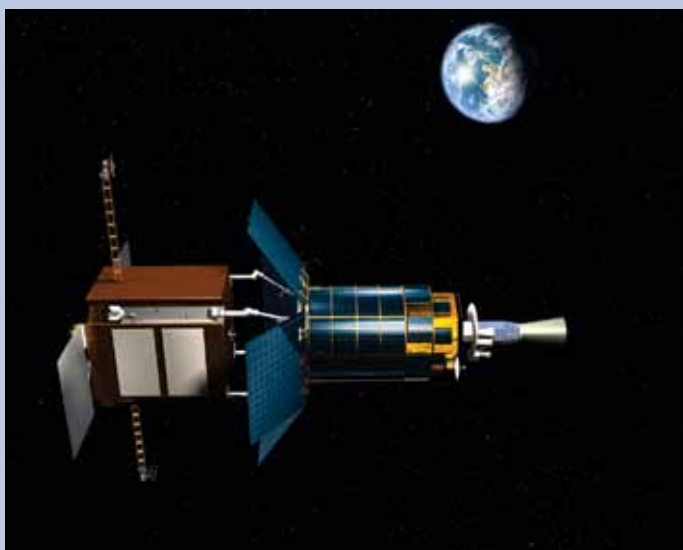
Figure 2.3 – Orbital Modification – This conceptual rendering shows a servicing spacecraft (left) mated with a customer spacecraft (right) to effect orbital modification – changing its orbital parameters to suit mission needs (see Notional Mission 1 in Appendix F).
