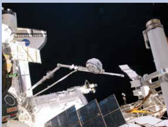
Figure 1.9 – ISS SSRMS Installing Cupola – In the grasp of the Canadarm2, the Cupola is relocated from the forward port to the Earth-facing port of the International Space Station’s newly-installed Tranquility node. NASA astronauts Terry Virts, STS-130 pilot; and Kathryn Hire, mission specialist, moved the Cupola, operating the station’s robotic arm from controls inside the Destiny laboratory. Also visible are a Soyuz spacecraft, the (space shuttle) Remote Manipulator System and portions of space shuttle Endeavour. This operation is a dramatic demonstration of the results of humans and robots working cooperatively.
