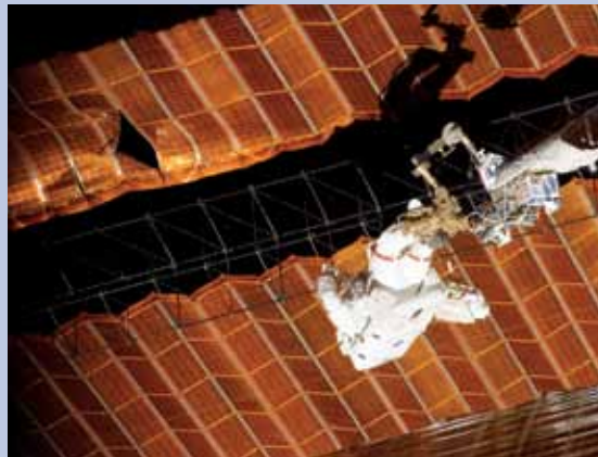
Figure 1.10 – ISS Solar Array Repair – While anchored to a foot restraint on the end of the Orbiter Boom Sensor System (OBSS), astronaut Scott Parazynski, STS-120 mission specialist, participates in the mission’s fourth session of extravehicular activity (EVA) while space shuttle Discovery is docked with the International Space Station. During the 7-hour, 19-minute spacewalk on November 3, 2007, Parazynski cut a snagged wire and installed homemade stabilizers designed to strengthen the damaged solar array’s structure and stability in the vicinity of the damage. Astronaut Doug Wheelock (out of frame), mission specialist, assisted from the truss by keeping an eye on the distance between Parazynski and the array. Once the repair was complete, flight controllers on the ground successfully completed the deployment of the array.
